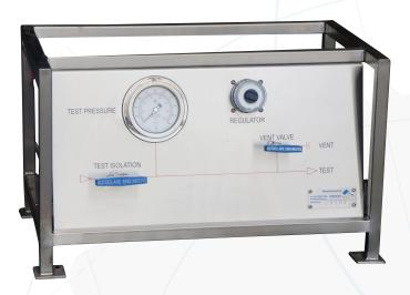
Trident Australia Hydrostatic Pressure Test Unit incorporating a choice of Haskel GSF Series pumps available in ratios from 12:1 to 100:1 for pressures to 11,500 psi.
